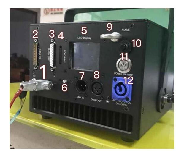
No.1: 9 pin Remote and key, if you want to make the laser work, the key must "on" and the 9pin remote must insert the 9pin interface.
